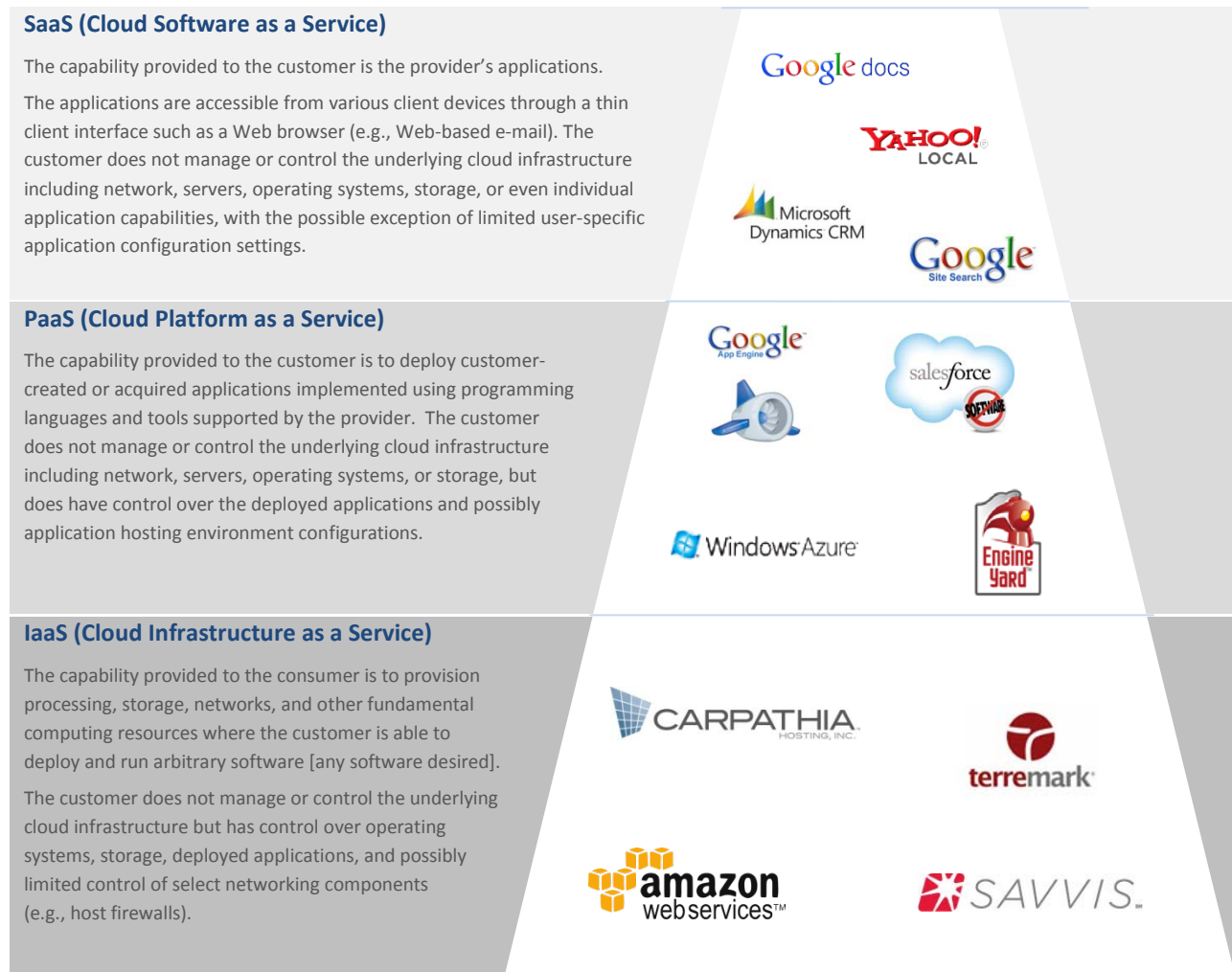
FIGURE 1: CLOUD COMPUTING SERVICE MODEL DESCRIPTIONS AND A SAMPLING OF CLOUD PROVIDERS
